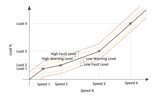
Offset from the expected Load line, 4 additional lines are calculated. These are the Warning and Fault detection thresholds. The deviation from normal behavior is determined by the **High Fault Level**, **High Warning Level**, **Low Warning Level** and **Low Fault Level** parameters.
